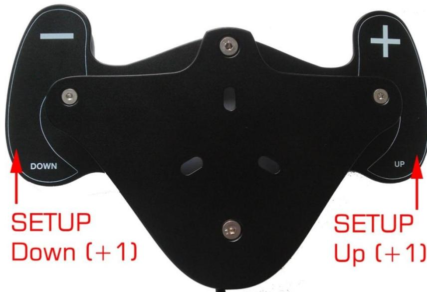
The Servomotor displays the actual selected Setup when changed by moving the lever 1x (Setup 1) .... 5x (Setup 5, default) ... 10x (Setup 10):
